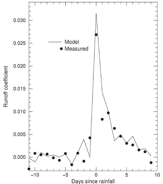
Fig. 9. Daily runoff coefficients derived from Fourier analysis of rainfall and discharge data (both measured and model). The non-zero values for days  $-11$  to  $-1$  (should be zero as these are days before rainfall) is due to the error introduced in assuming that only the rainfall and discharge are time dependent. The scatter in these values gives an estimate of the noise level throughout the curve.
