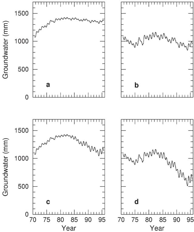
Fig. 13. Model mean groundwater storage in mm: (a) no natural loss and pre-network pumping; (b) with natural loss and pre-network pumping; (c) no natural loss and post-network pumping; (d) with natural loss and post-network pumping.
