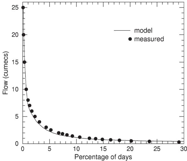
Fig. 8. Model and measured flow duration curves.
